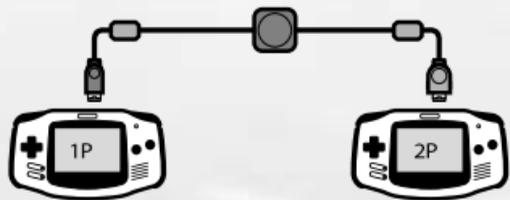
\*The system with the smaller plug connected is the 1P side.
